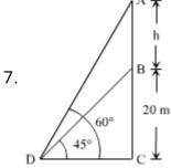
Let BC be the building, AB be the transmission tower, and D be the point on the ground. In  $\Delta BCD$ ,
