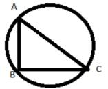
Since AB is perpendicular to BC, therefore ABC is a right-angled triangle right angled at B. As clear from the figure, AC would act as the diameter
