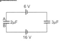
Here, 2  $\mu$ F and 3  $\mu$ E capacitors are connected in series. Their equivalent capacitance is,  $\frac{1}{C_S} = \frac{1}{2} + \frac{1}{3}$  or  $C_S = \frac{6}{5}\mu F$
